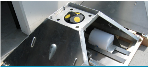
An XR and battery pack installed in an optional trawl-resistant mount.
