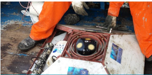
Pyramidal housing protects the Argonaut-XR from damage in busy ports, as shown here in Brazil.*
